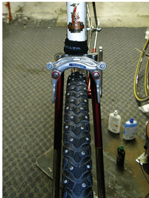
The Schwalbe Marathon Winter tires have studs in the center and on the edges, 240 in all.
